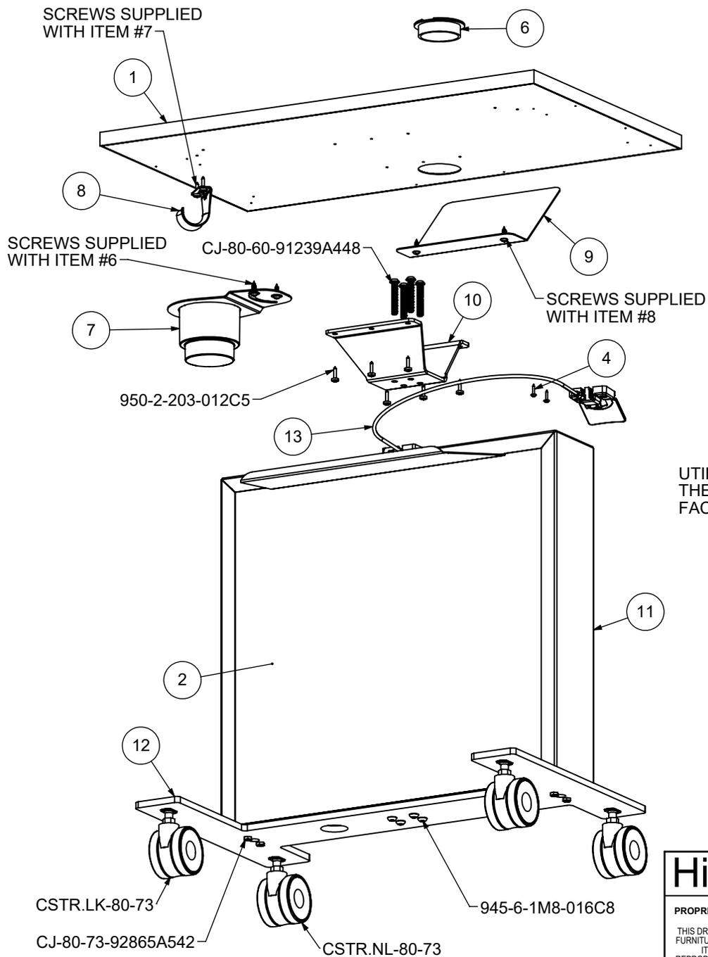
UTILIZE ITEM 5 (NOT SHOWN) TO SECURE THE ACTUATOR CABLE TO THE LOWER FACE OF THE TABLE TOP
