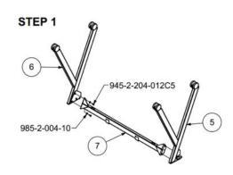
Step 1. Use Screw #945-2-204-012C5 and Washer #985-2-004-10 to attach the Support Beam to the Legs
