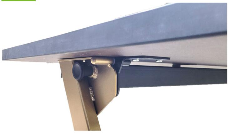
Step 4. Twist Plunger to unlock on both ends of the table. With the plungers not engaged, the base will not flush to the tabletop. Push the table legs until they allow the plungers to lock on both sides.
